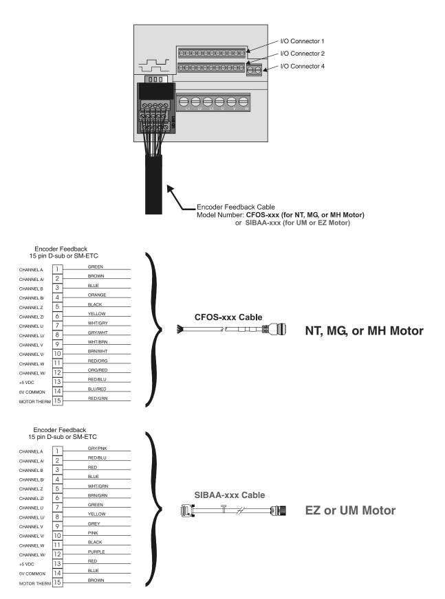
Figure 3: Motor Feedback to Unidrive SP Connection Diagram
